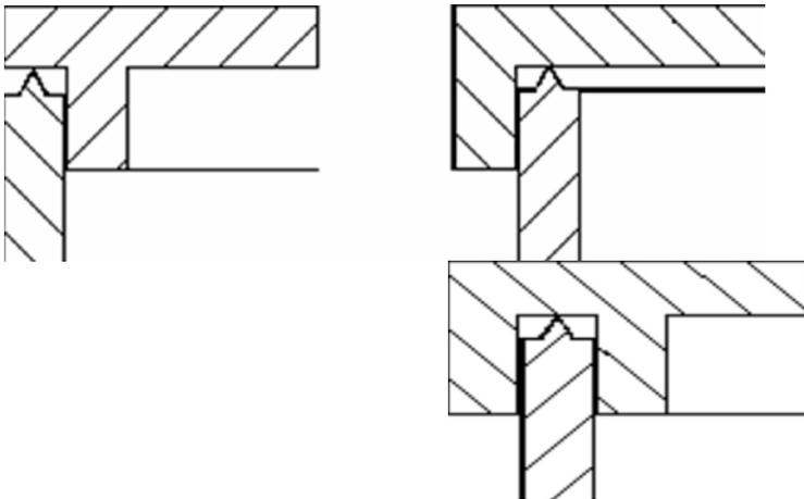
A feature that is shown in these joint alignment pictures is the molded-in triangular shape of material called an energy director. This molded-in triangular ridge of plastic is very effective at reducing the cycle time to achieve a weld and in compensating for non-uniform wall surfaces. The energy director design has been used for years as a means of focusing the energy to improve weld strength and reduce cycle time.
