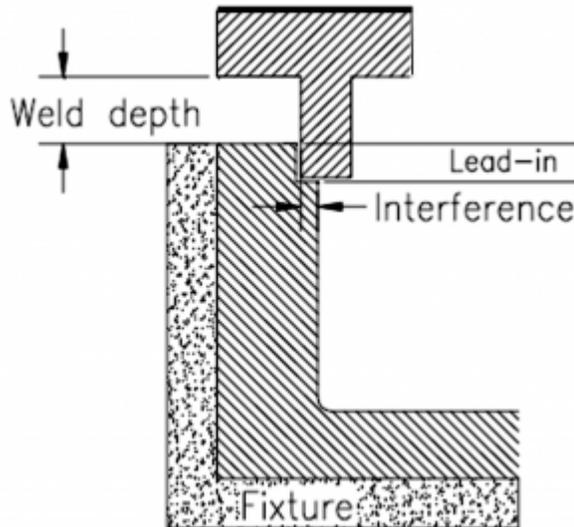
Guidelines for Shear Joint Interference
