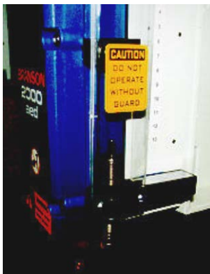
PAT HydroSnubber on Branson 2000 ultrasonic welder
