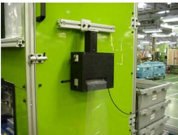
*PAT Film Winder mounted to the outside of an assembly unit*
