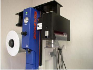
*The PAT Protective Film Winder stands apart from its competitors in "White Room" applications where, as opposed to compressed air driven systems, its electronically controlled mechanical drive assembly releases no contamination into the atmosphere, thus maintaining white room integrity.*
