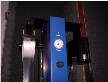
*PAT Film Winder installed in a Branson Sound Enclosure*
